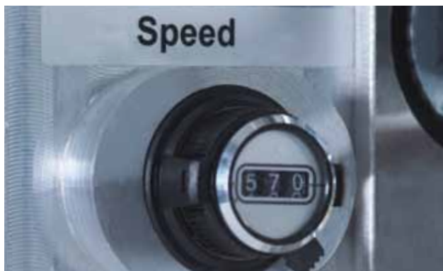
Precise speed adjustment via multi-ratio potentiometer.
