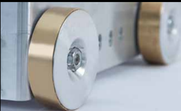
Chassis with 4 magnetic wheels, for perfectly straight tracking.
